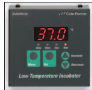
Digital display shows temperature readings and active alarm.
