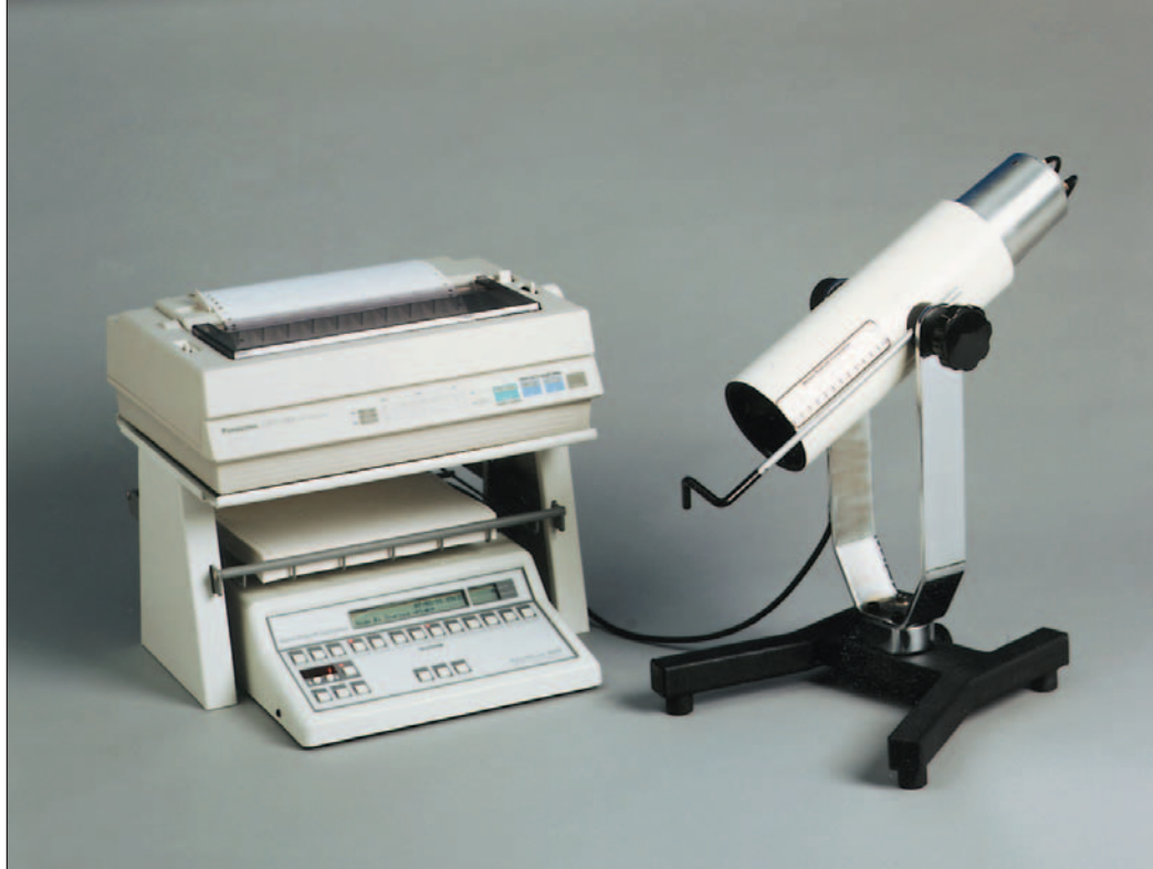
▲ The Tabletop System is self-contained, requiring a minimal amount of counterspace. The 256 channel MCA is built into the Atomlab 930. Shown with optional printer shelf.
